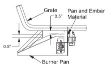
Figure 24 - Pan and Ember Material Clearances
